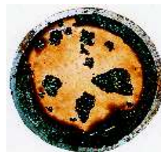
Sample after 60 hours incubation with Para-Bac/S at 25,000 ppm.
