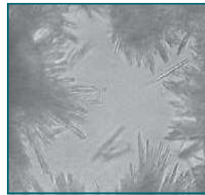
Untreated calcium sulfate scale. Notice large crystals.
